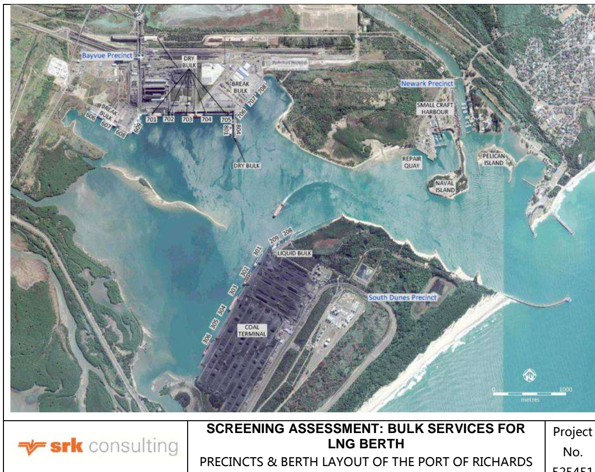
Figure 4-1: Precincts and berth layout of the Port of Richards Bay (extracted from the National Ports Plan 2016 Update)
